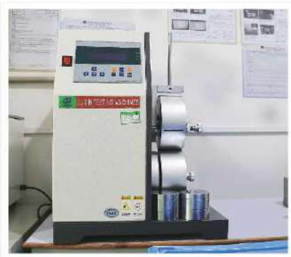
Velcro Lifecycle Testing
