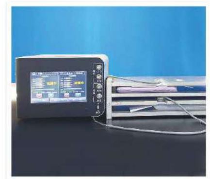
Bladder Lifecycle Testing
