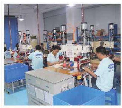
RF Welding Process
